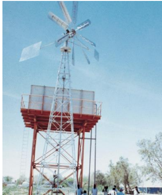
Figure 5. Locally-manufactured wind pump installed at kilo 8 site.
